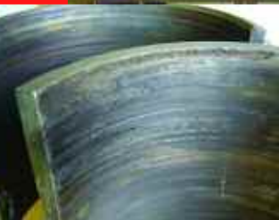
damaged white metal bearings after gearbox strip
